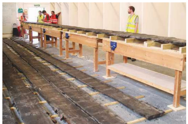
Once dry, however, the planks emerged straight, split-free, and astoundingly flat. When laid on this platform with a stick every 600mm, they touched at every single point!
